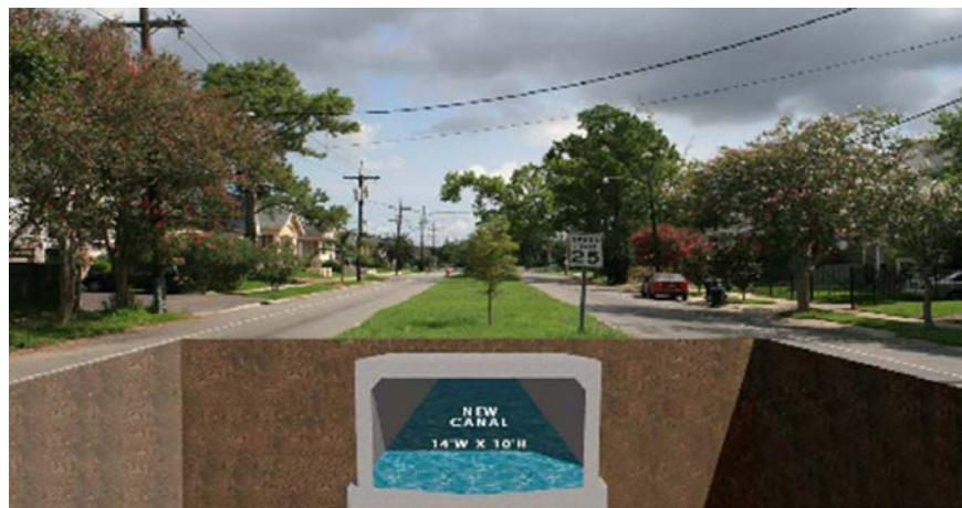
Pictured above: Conceptual image of what the new underground concrete box culvert will look like.
